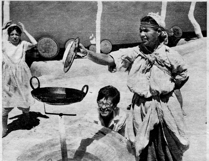
Mrs. Hammouche Abdeslem, wife of a commune leader, pours oil into a black frying pan that is supported over four concentric rings of board covered with aluminum foil. The foil reflects sun's rays onto pan.
