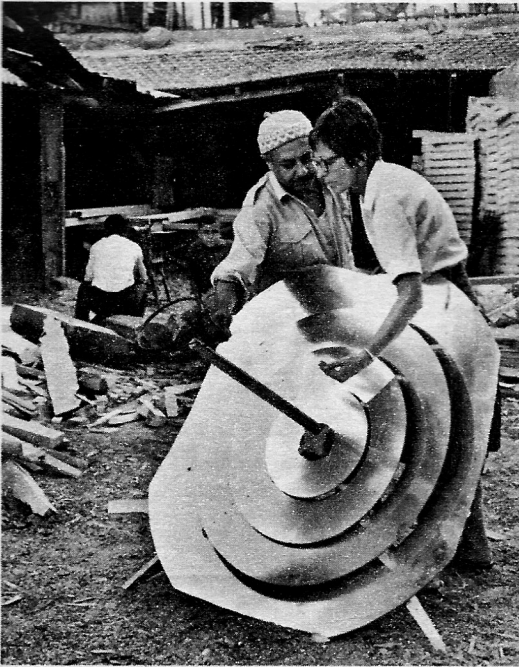
Moroccan carpenter Abderrahman Bouchareb and Virginia Hazzard examine a solar cooker that Bouchareb makes in his shop.
